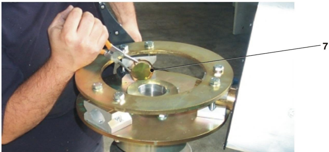
Figure 2-4: Blade assembly for blades of AP impellers.
